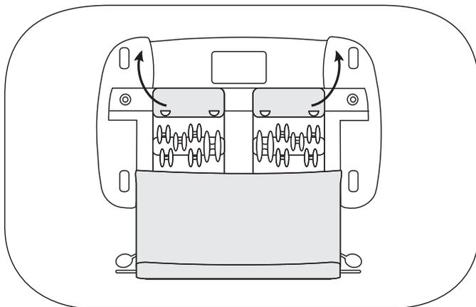
3. Take 4 remaining loops off the plastic shafts, located in front of the massage mechanism (see the picture to the left).
